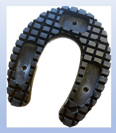
• Clamp your farrier prepared/fitted horseshoe into the Bolt-On Boot and, using either the ¼" drill bit or a ¼" shank center drill, scribe your hole locations from the Bolt-On boot to the farrier prepared/fitted horseshoe. If using the ¼" drill bit, be careful not to plunge past the tip of the drill bit as the next step will require drilling a hole smaller than ¼".
