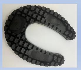
Mark your desired hole locations on the Bolt-On boot. Drill ¼" thru holes in the Bolt-On boot soles like as shown on the right. We recommend using a center drill or a punch before the ¼" drill. Be sure to drill through enough to make a relatively clean hole through the rubber located on the top side of the Bolt-On boot sole.
